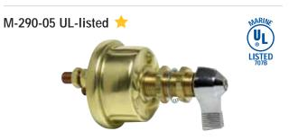
Brass case. Silver laminated contacts. Chrome-plated diecast lever. Brass mounting stem 3/4" -16 thread 1 13/32" (46.1mm) long. Fits panels through 15/16" (23.8mm) thick. Two 3/8" -24 and two 10-32 studs. Labeled UL 707B.
