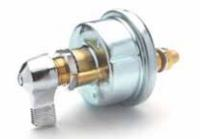
Diecast lever. Plated steel case. Silver-laminated contacts. Brass mounting stem 3/4" -16 thread 17/32" (13.5mm) long. Fits panels through 1/4" (6.4mm) thick. Two 3/8" -24 and two 10-32 studs. O-ring seal in the operating shaft, and gasketsealed terminal insulator.
